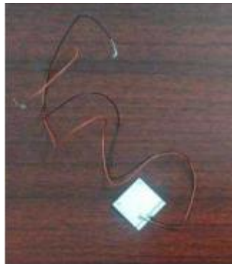
Figure 2 Piezoelectric actuator and sensor
